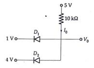
If the diodes  $D_1$  and  $D_2$  are ideal, then the value of  $V_0$  and  $I_0$  are respectively
