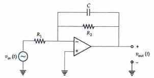
If  $V_{in}(t) = 2e^{-2t} u(t)$  V and  $V_c(0) = 0$ , then  $V_0(t)$  is
