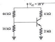
The value of the collector-to-emitter voltage  $V_{CE}$
