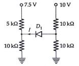
If the cut-in voltage of the diode  $D_1$  is equal to 0.7 V, then the value of current flowing through the diode is
