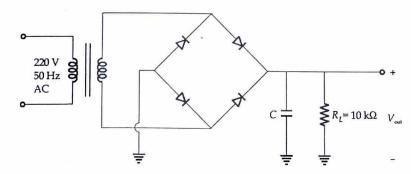
The value of capacitor C to maintain the peak to peak ripple voltage as 1% of maximum value of input voltage ( $V_{max}$ ) is
